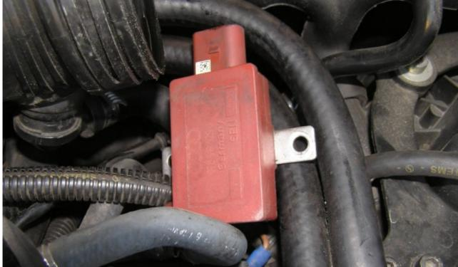
6. Open EGT electronic housing. There is no uniform recipe to do this. Sensors could be levered near connector, but depending on how it is glued by the producer, sometimes it's easier, sometimes harder to open it.
