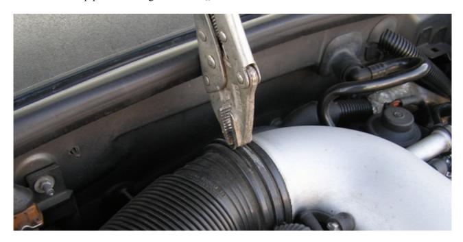
4. Remove the "Y" air distributor. To do this, unscrew three M6 screws (1, 2, 3), disconnect the pressure limiting valve (4) and relase two clamps located near DV's (5 and 6). Then remove the "Y" air distributor. After this operation, two EGT's are easily accessible (in AJK, AGB engines EGT's are placed symetricly to the longitude motor axis, in ARE, BES both EGT's are on the right side of the engine in the same place)
