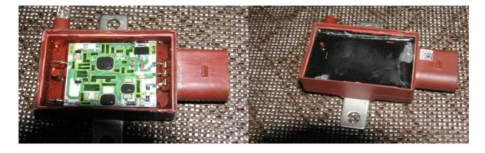
8. After removing the protective substances desolder (or cut), old electronics and disassemble it. Be careful not to damage electrical connections.
