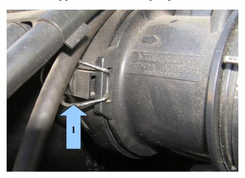
3. Remove the pipe connecting MAF with "Y" air distributor.
